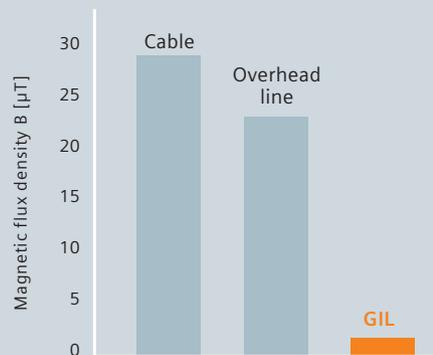
A comparison of the magnetic fields for different high-voltage transmission systems.
